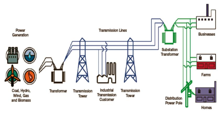
There are three distinct functions involved in moving power from its source to consumers; each plays a different role in a complete electric system.
