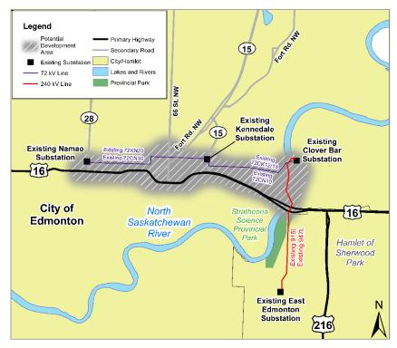
The shaded area in the map indicates the approximate area of the proposed transmission reinforcement and identifies the existing substations.
